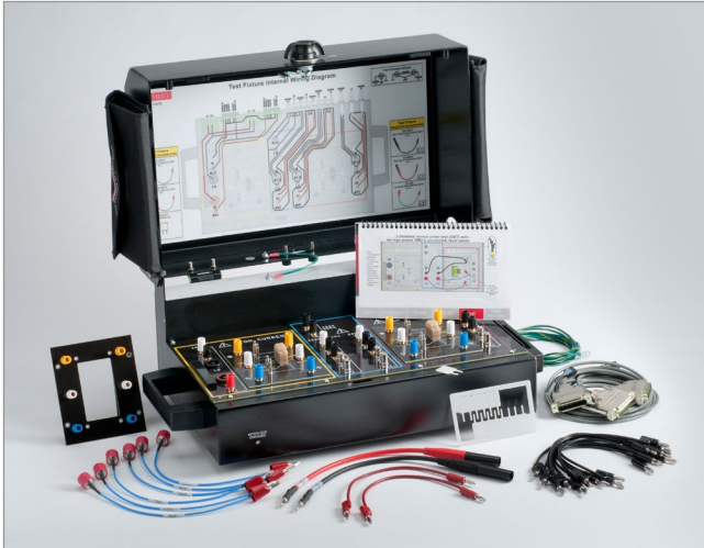
8010 High Power Device Test Fixture.
